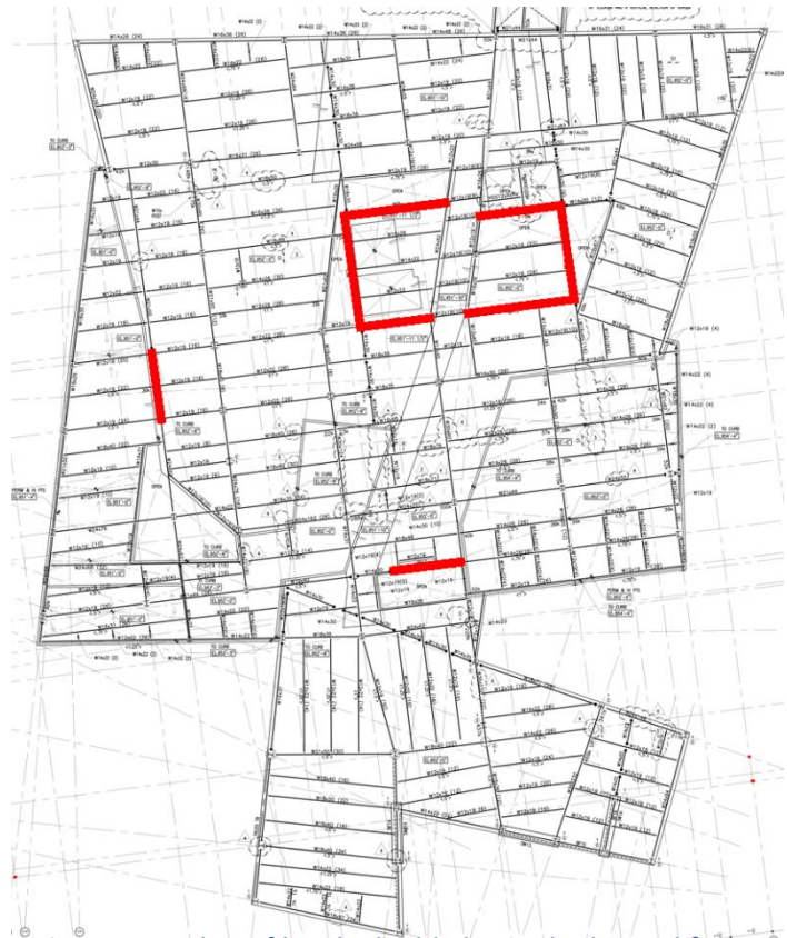
Figure 12 - Plan of level 6 highlighting the braced frames
