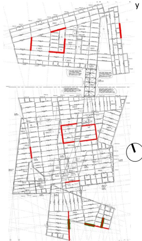
Figure 6 – Level 6 plan showing shear wall/braced frame layout
